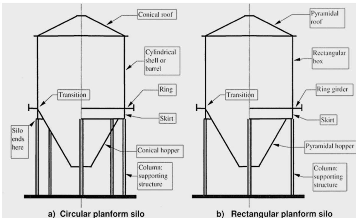
Figure 1: Terminology used in solid storage structure structures
