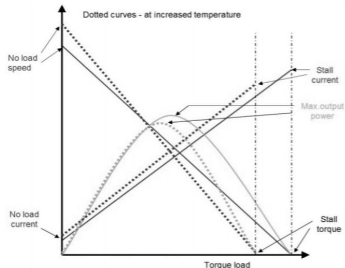
**Figure 3. Composite PMDC motor's characteristics, representing relationship of efficiency, torque, current, speed, and power for voltage at Nominal temperature Vs increased Nominal temperature (curtesy: Carryer, Kenny et.al)**
