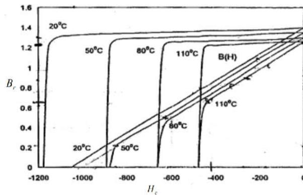
Figure 1 characteristics of Demagnetization in NdFeB (Neodymium Iron Boron) magnets at different temperatures
