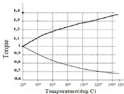
Figure 2 Applied torque against Required Torque Vs Temperature capability of PMDC motor
