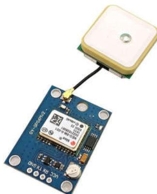
The NEO-6 module series is a family of stand-alone GPS receivers featuring the high-performance u-blox 6 positioning engines. These flexible and cost-effective receivers offer numerous connectivity options in a miniature 16 x 12.2 x 2.4 mm package. Their compact architecture and power and memory options make NEO-6 modules ideal for battery operated mobile devices with very strict cost and space constraints. The 50-channel u-blox 6 positioning
