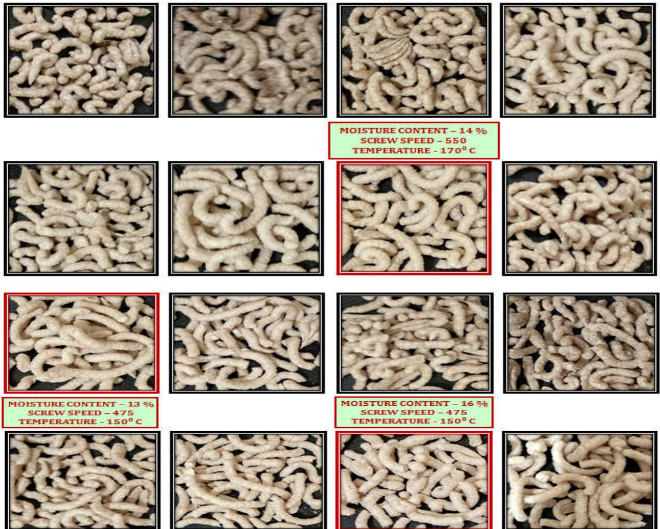
Figure 2: Glutinous rice based snacks extruded at different processing conditions
