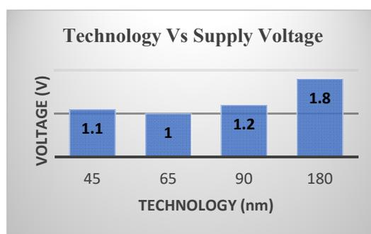
**Figure 1: Technology used vs supply voltage**
