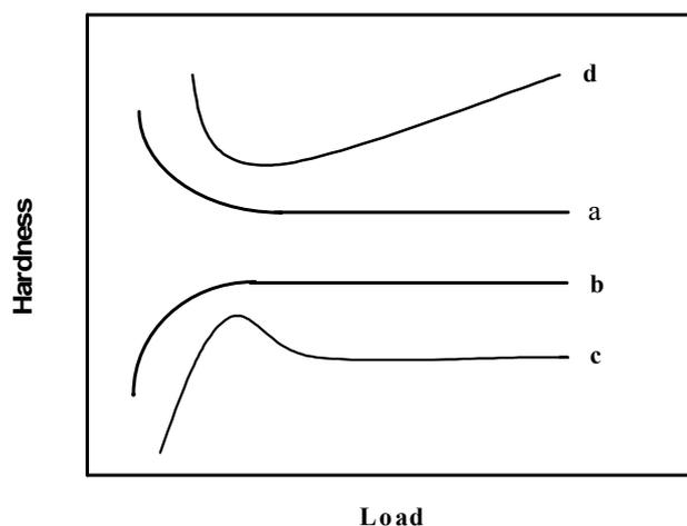
**Figure 1:** Types of load variation of hardness.
