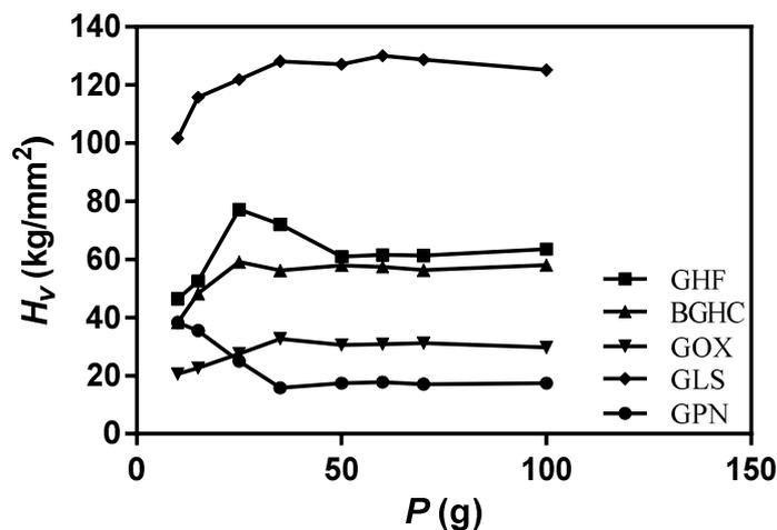
Figure 2: Load-hardness curves for the crystals under study.
