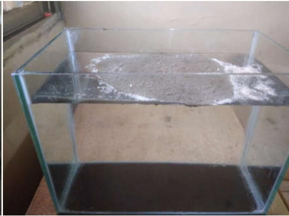
**Figure 2. Oil Layer With PVC Powder**
