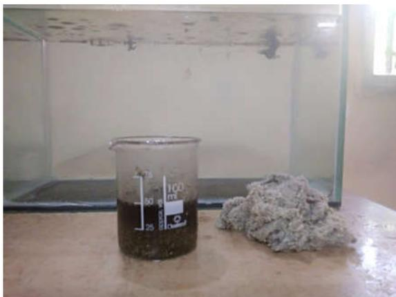
**Figure 31. Squeezed cotton releases absorbed oil in to beaker shows over 90 % removed.**
