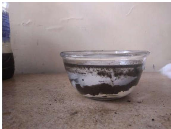
**Figure 28. Cotton -Tyre Powder Pushes Oil Down**
