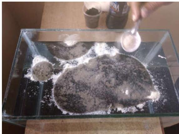
**Figure 13. PVC Powder Over Oil surface**
