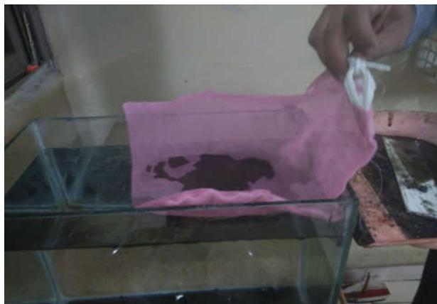
**Figure 5. Removing Oil Slab With Nylon Mesh**
