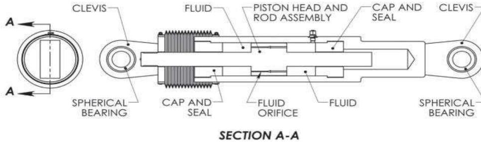
**Fig. 1 . Logitudinal section of FVD**
