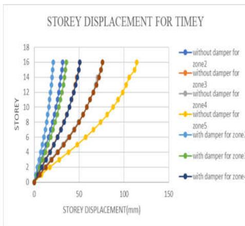
Fig. 14 : Storey displacement in y direction for time history method
