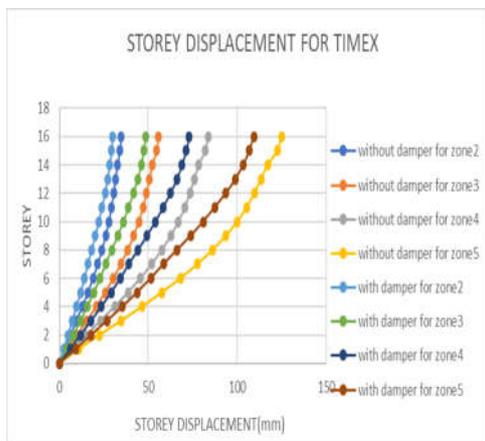
Fig. 13 : Storey displacement in x direction for time history method
