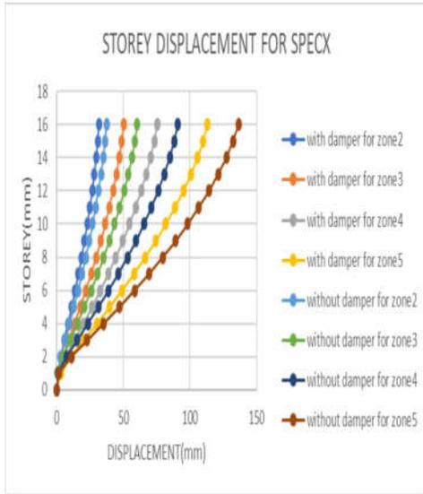
Fig. 11 : Storey displacement in x direction for response spectrum method
