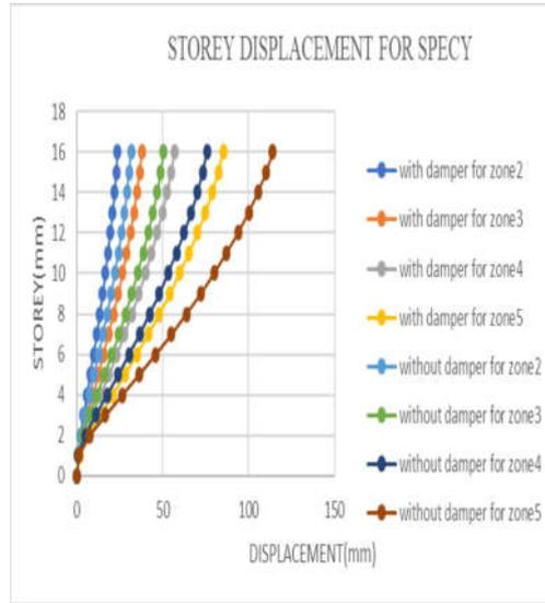
Fig. 12 : Storey displacement in y direction for response spectrum method
