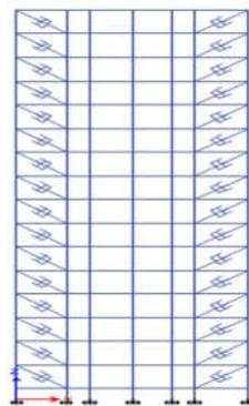
Fig. 5 : FVD at exterior corner Elevation
