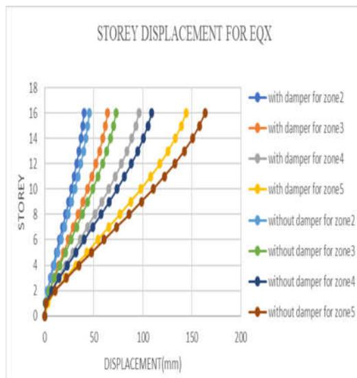
Fig. 9 : Storey displacement in x direction for static method
