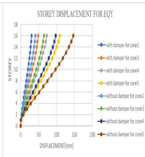
Fig. 10 : Storey displacement in y direction for static method
