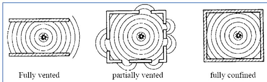
Figure 3. Confined explosion
