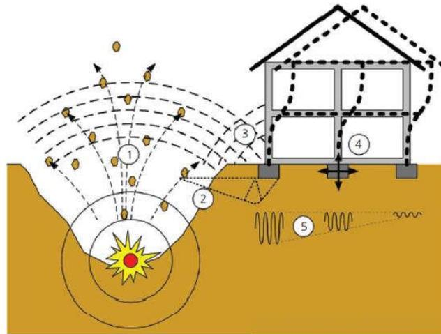
Figure 4. Damage patterns due to underground explosion
