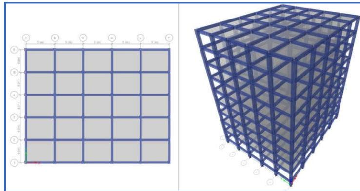
Figure 6. Plan and 3D view of ETABS model
